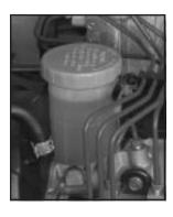
You can check the brake fluid without taking off the cap.
